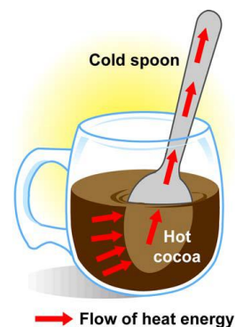
Figure 11.11: Heat flows by conduction from the hot cocoa into, and up, the spoon.
